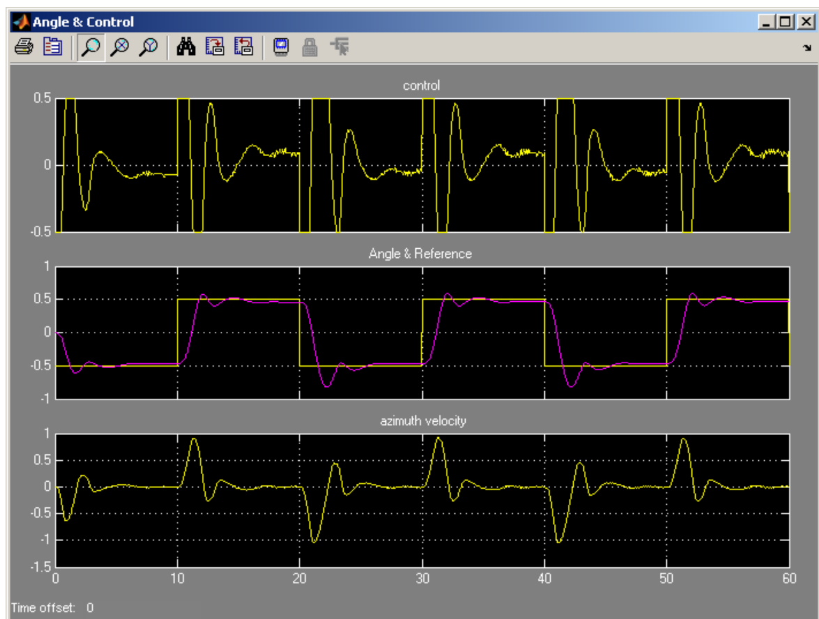
Fig. 7.10 Results of PID azimuth control
