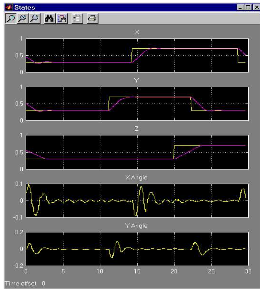
Fig. 6.23 The X, Y, Z positions and X, Y angles visible in the States scope
